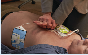
Real CPR Help® assists rescuers during adult rescues with real-time feedback on chest compression rate and depth.
